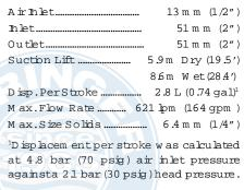
Example: To pump 197 lpm (52 gpm) against a discharge head of 4.8 bar (70 psig) requires 5.5 bar (80 psig) and 75 Nm  $^3/h$  (44 scfm) air consumption.
