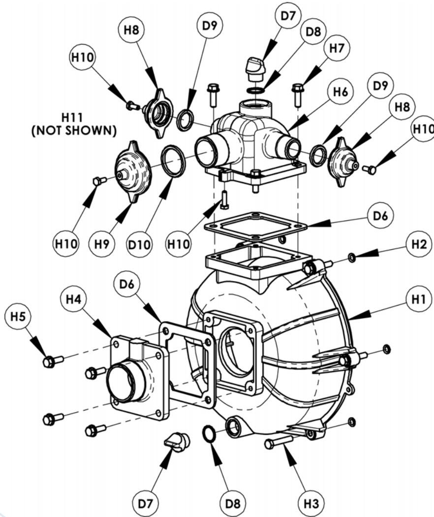
Figure 2 - Repair Parts Illustrations - Casing
